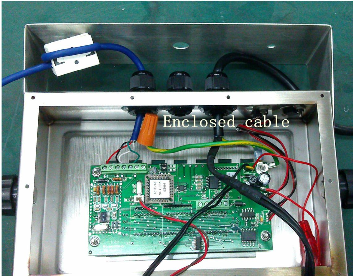
The TI-500E-SS indicator contains a connection terminal on the main board assembly for connection to the load cell cable. . **NOTE:** 6-wire connection is optional.
