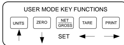
4. After setting the exact value, press the NET/GROSS key to save the ID Number value. The display will show "**SET**" momentarily, and then revert back up to A8.
