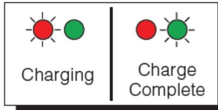
To prolong battery life, disconnect the external battery charger from the unit when charging is complete (Green LED).
