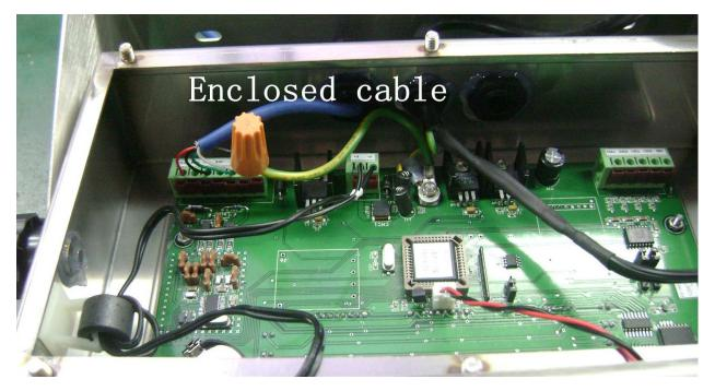
The TI-1520 indicator contains a connection terminal on the main board for connection to the load cell cable. Connect your shielded load cell cable (not included) to the appropriate terminal on the main board. **NOTE**: 6-wire connection is optional.
