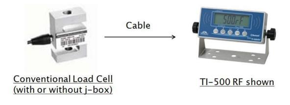
When sold with an external TI-500 RFTM (Radio Frequency Transceiver Module) and an optional wireless radio, your TI-500 RF series indicator is transformed from "wired" to cable-free. This configuration is depicted in the following diagram:
