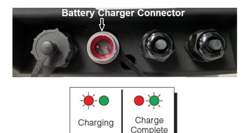
To prolong battery life, disconnect the external battery charger from the unit when charging is complete (Green LED).
