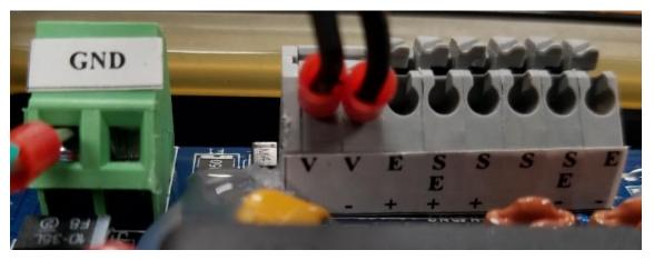
**NOTE1**: Use F11 to configure for 4-wire or 6-wire load cells **NOTE2**: Pins 1 and 2 are for DC power input (V+ and V– respectively) ... **NOTE3**: There are two configurations for J1, as shown above, and differing only in the location of the load cell shield wire connection (GND)
